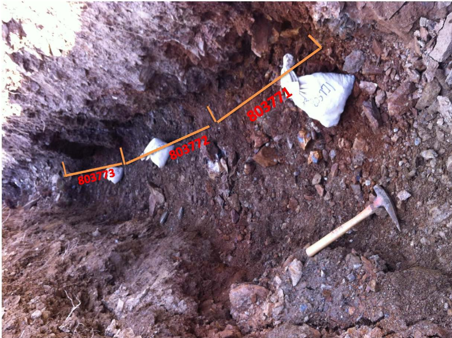
Figure 1: 6 meter chip sample grading 6.99 gpt gold from backhoe trench on the Coffee Dome prospect, Fairbanks Mining District, Alaska. Geochemistry from samples is included in Table 1.
